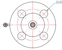
FLANGE DIMENSIONS AND WORKING PRESSURES ARE AS STATED IN ASME B16.5
