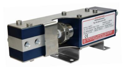
The Air Pilot Switches are designed to switch a pneumatic signal and are used to shutt-on or shut-off MAXIMATOR pumps and boosters upon achieving a desired outlet pressure. The Air Pilot Switches are available in various pressure ranges for outlet pressures from 10 to 1,000 bar. The switch does contains both functions "Air to open" and "Air to close".
