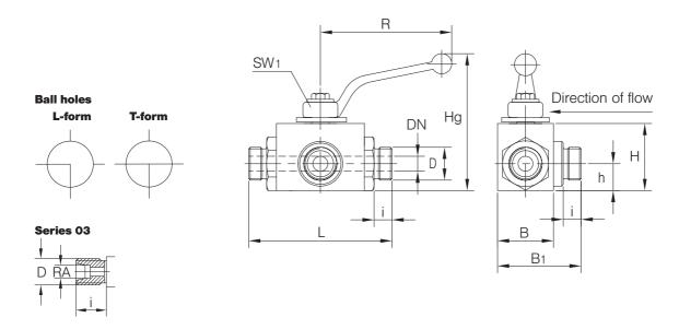
Series 02 (for non-soldering compression fittings with cutting ring DIN 2353, light-duty series)
