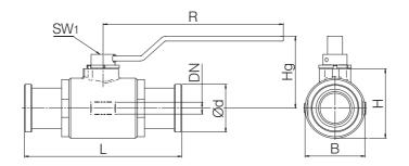
Series 68 (Connections on both sides with pipe sockets for SAE half flanges 3000 psi)
