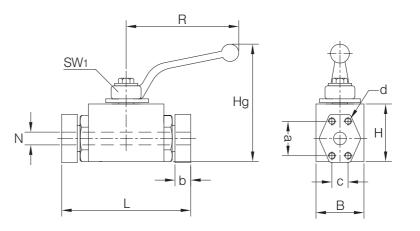
Series 68 (swivelling SAE flanges on both sides 3000 psi )
