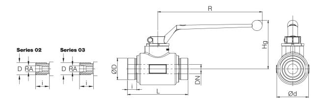
Series 02 (for non-soldering compression fittings with cutting ring DIN 2353, light-duty series)
